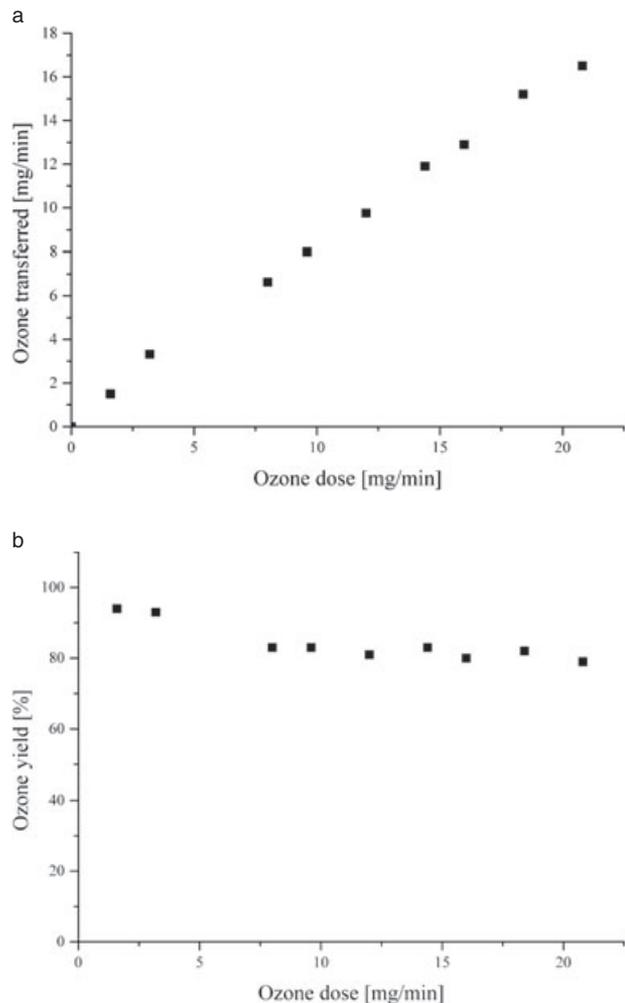
**FIG. 3.** (a) Transfer and (b) total yield of ozone by using GED L001 and the ozone generator B.
