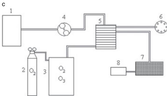
**FIG. 1.** GED L001 (a) the external aspect, (b) the cross section, and (c) a schematic diagram of the circuit (1, saline solution; 2, oxygen supply; 3, ozone generator with photometer; 4, peristaltic pump; 5, GED; 6, sample collector; 7, silica gel trap; 8, ozone destructor).
